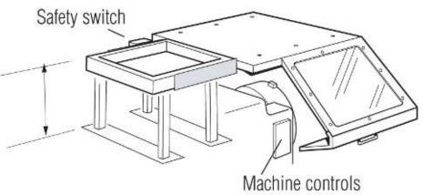
150-250mm adjustable height standard (made to order over 250mm height)
