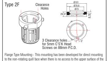
to the non-rotating quill face when there is no access to the upper surface of the quill flange and necessitates tapped holes being provided in the face of the quill flange for fixing purposes.
