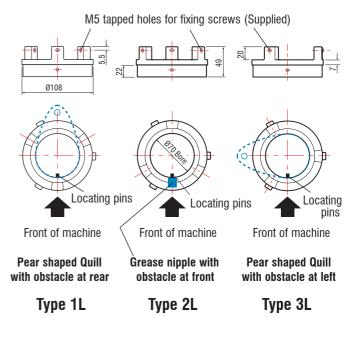
The lugs on the fixing collar are bored out to a maximum of Ø96.00mm. The collar is attached to the fixed quill by adjusting the fixing screws to suit the required diameter.
