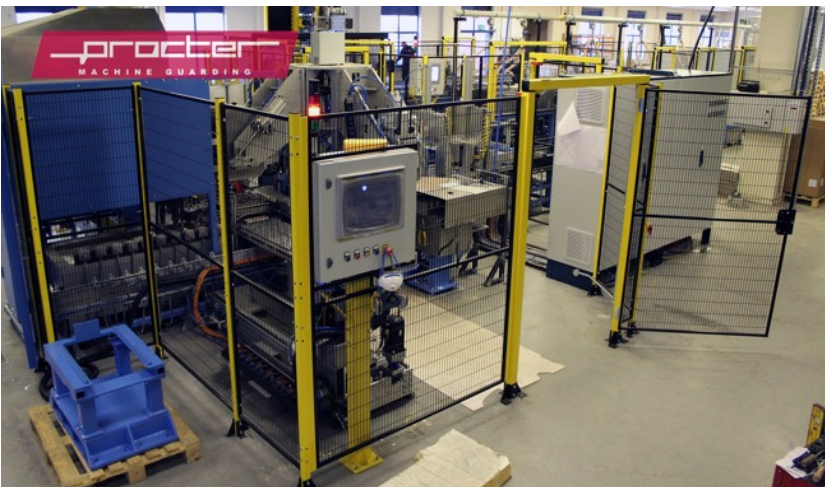
The enclosure including custom cut out for control panel
