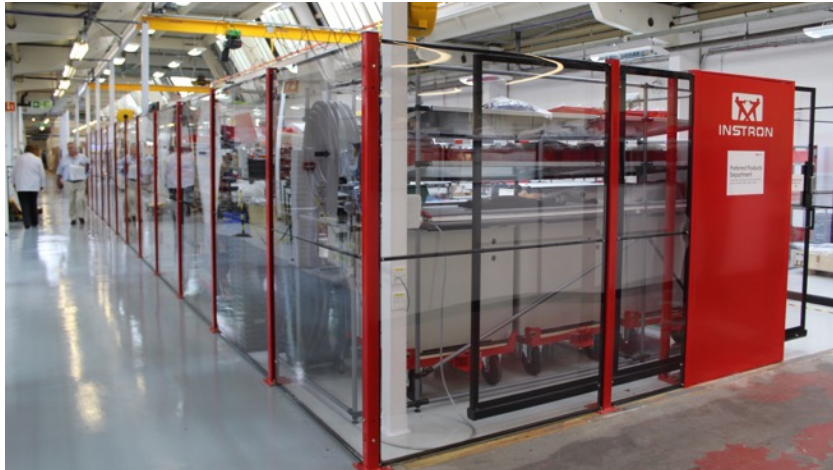
Bespoke polycarbonate guarding with company logos added
