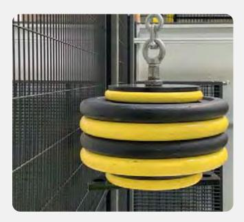
Mass release height from the ground (mass load center): **h0** = 3,060 m Mass impact height from the ground (mass load center): **h1** = 1,420 m
